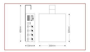
The PDU distributes DC power (24V) and the DMX data signal through the XLR4-pins female to a maximum of 24 Xpress Colour Scrollers.
